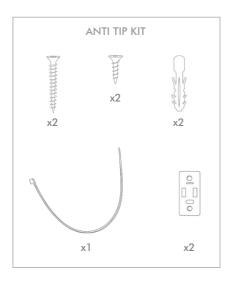
Please use the anti tip kit provided for safety. Please ensure the correct fittings are used for the chosen wall substrate:
